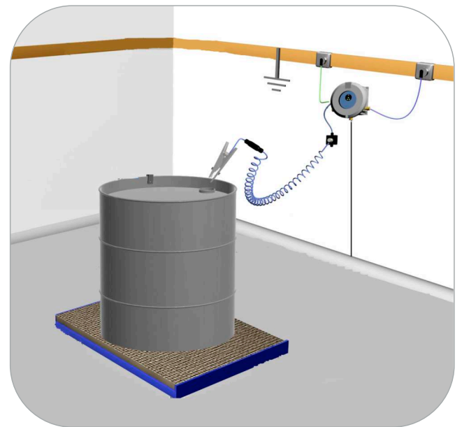
Example of correct grounding technique for a static dissipative drum
